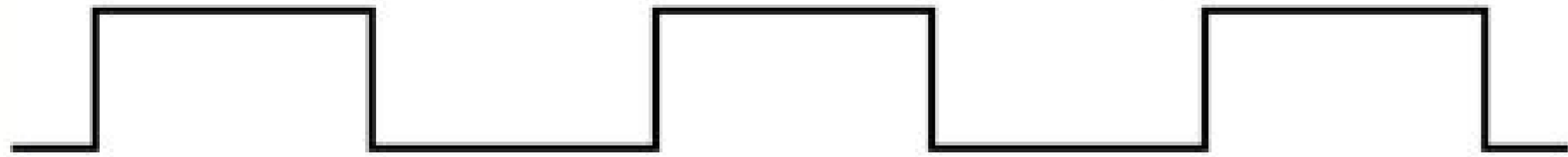
1a: 1:1 mark-space ratio (50% duty cycle)
