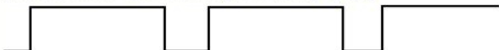
1b: 3:1 mark-space ratio (75% duty cycle)
